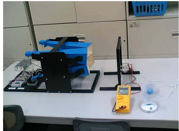
Fig.9. Test devices for wireless power transmission for electric vehicles
